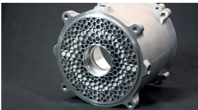
FIGURE 2: Additively manufactured housing of a PMSM with integrated cooling and lightweight structures out of AlSi10Mg.
