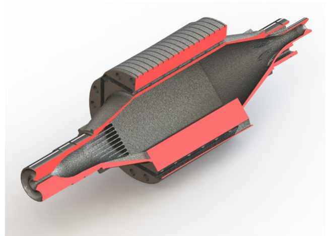
FIGURE 1 Sectional view of the optimised AM rotor
