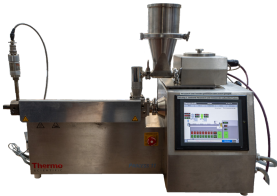
FIGURE 1 The Thermo Fisher Process 11 mini twin-screw extruder is used for the compounding process
