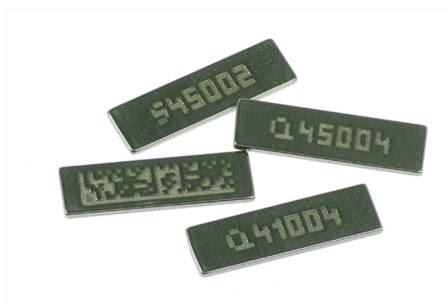
FIGURE 2 Individual markings directly produced during Selective Laser Melting
