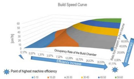
Figure 34: Build speed curve with regards to occupancy rate of the build chamber and the support ratio
