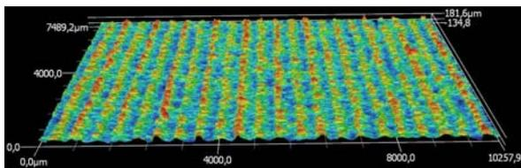
Figure 42: Exemplary 3D measurement of a 15° tilted surface. The shown field of view is used for the different analysis methods
