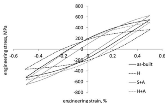
Figure 26: Half-life hysteresis loops for SLM processed IN 718. Tests were carried out at 650 °C with a total strain amplitude of  $\Delta\epsilon/2 = \pm 0.5\%$
