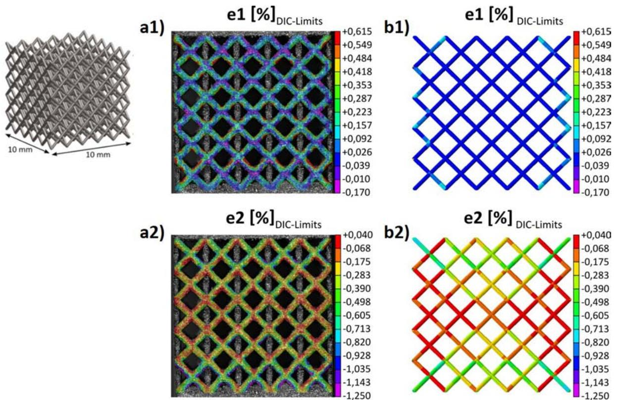
Figure 37: Local strain distribution of the fcc lattice structure under compressive load (a) maximum principal strain  $e1$  and minimum principal strain  $e2$  for the DIC; b) Simulation
