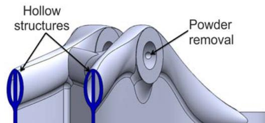
Figure 47: Bracket design with internal structures
