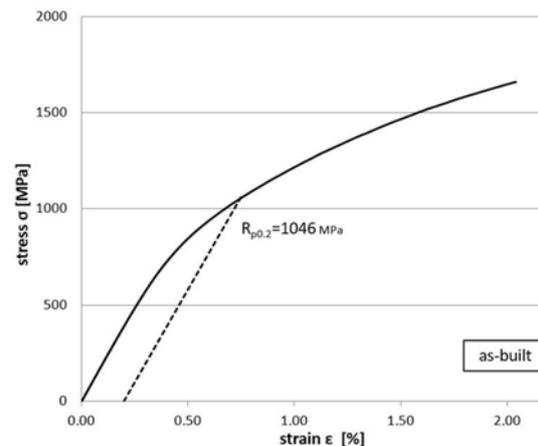
Figure 24: Results of tensile tests on H13 specimens
