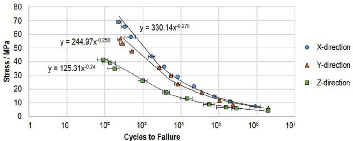
Figure 19: S-N curve for untreated Ultem 9085
