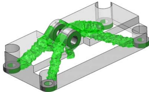
Figure 46: Topology Optimization of the bracket
