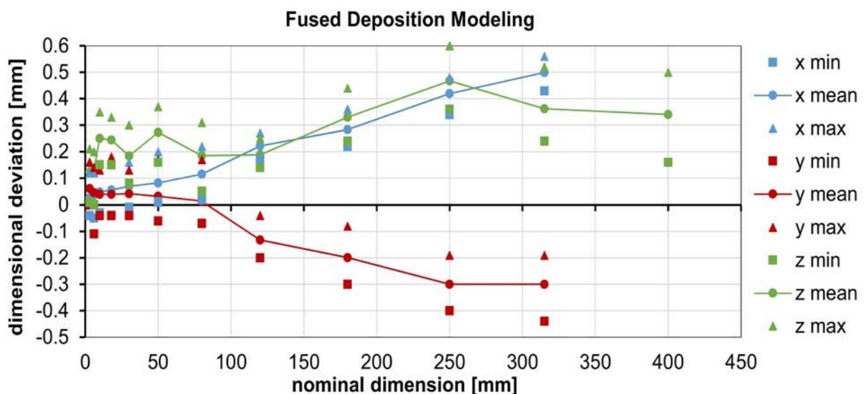
Figure 11: Maxima, minima and mean values of the occurring dimensional deviations for different nominal dimensions and alignments (x,y,z)
