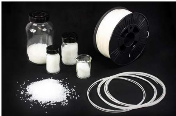
Figure 38: PA6 granulate is extruded into monofilaments
