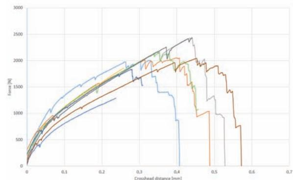
Figure 7: Force-distance diagram of support-structure (block) tensile specimen
