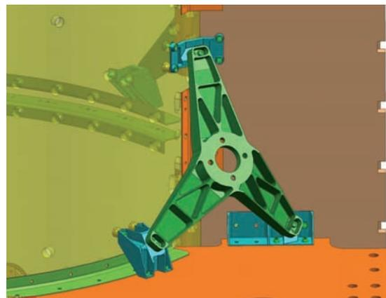
Figure 56: Traditional design of Reaction Wheel Bracket mounted in Exo Mars satellite
