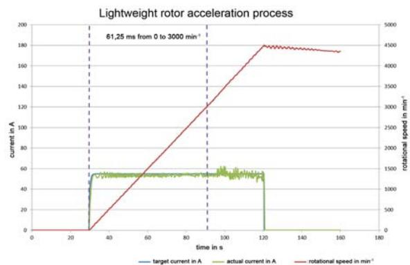
Figure 55: Results of the motor characteristics investigations.
