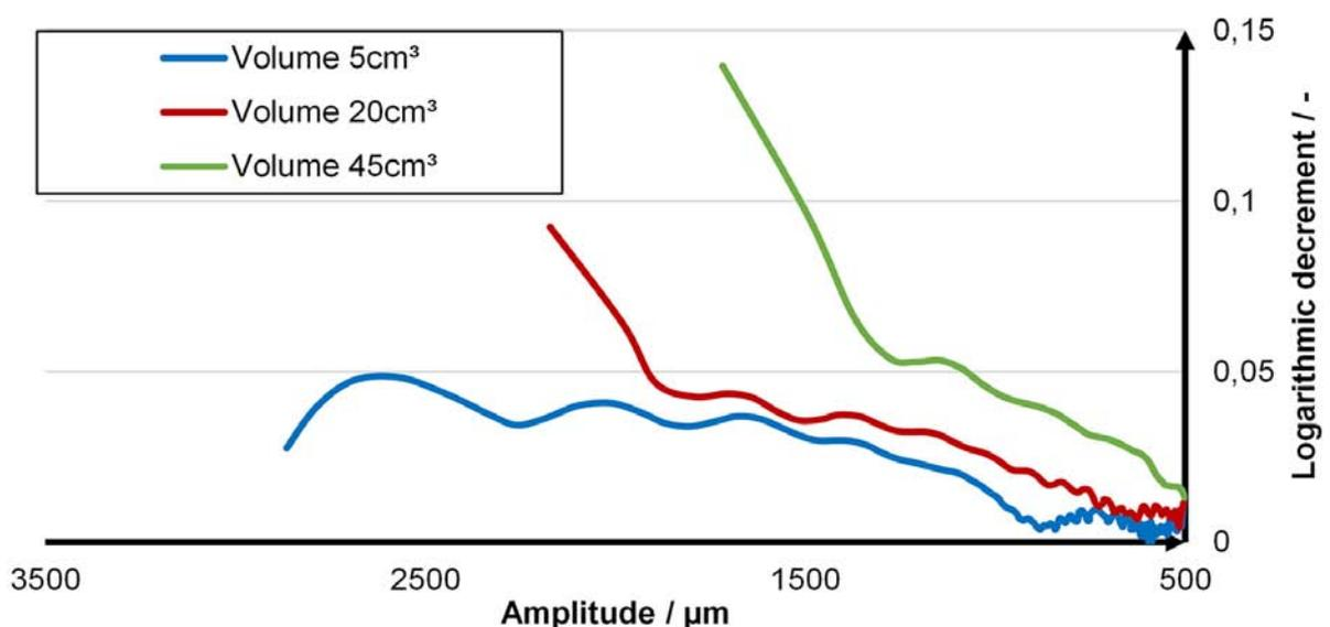
Figure 6: Damping behavior of different cavity volumes (LBM)
