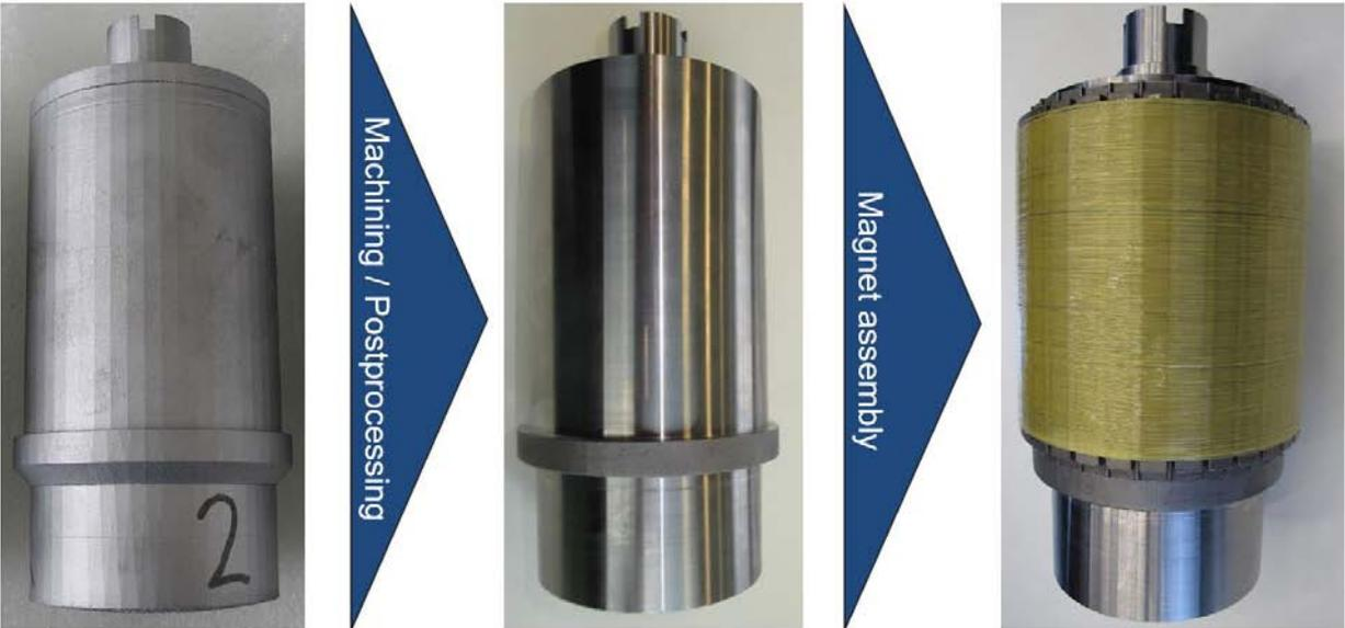
Figure 25: Additive manufactured rotor and after treatment
