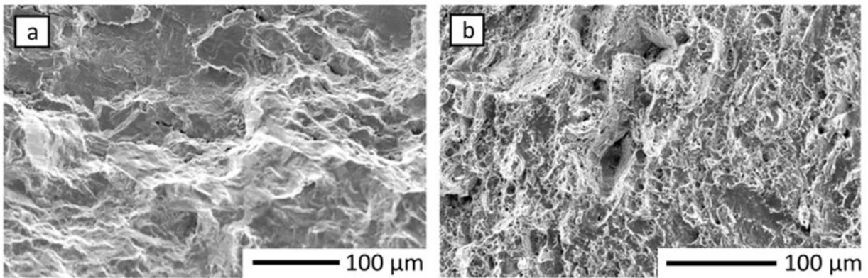
*Figure 27: SEM images of the fracture surfaces after LCF testing ( $\Delta\epsilon/2 = \pm 0.35\%$ ) at 650 °C in the as-built (a) and H (b) condition. The images were taken from the fracture surface showing instable crack growth*
