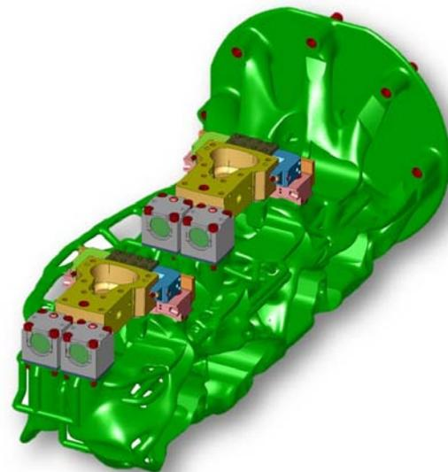
Figure 49: Topology optimized clamping device
