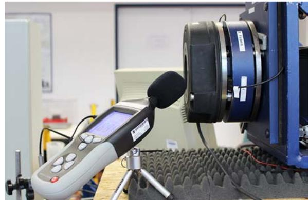
Figure 50: Test rig used for sound pressure level tests
