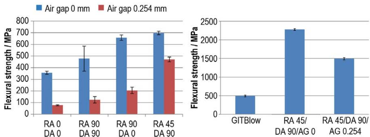
Figure 23: Flexural strength levels for different filling parameters (left) and flexural strength levels for the unreinforced GITBlow part and the reinforced GITBlow part (right)
