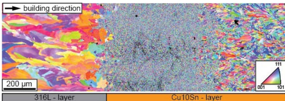
Figure 67: Color-coded orientation map of the functional graded multi-material consisting of 316L and Cu10Sn at an interface area.
