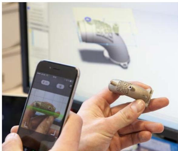
Figure 61: Using additive manufactured QR Codes for product verification
