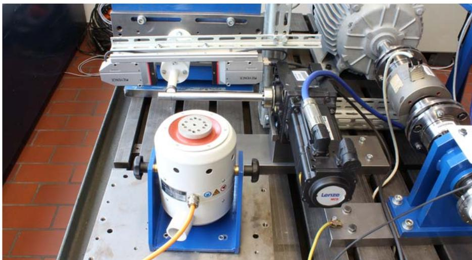
Figure 64: Developed test rigs for the investigation of additive manufactured damping structures
