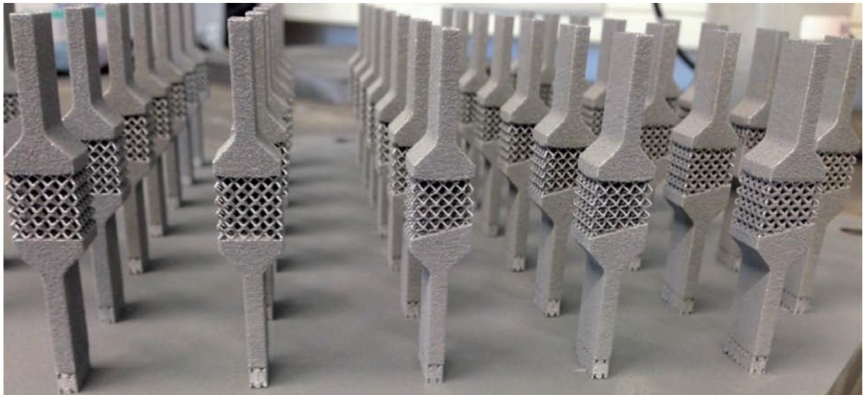
Figure 9: Building plate with different samples for the investigations on standard lightweight structures
