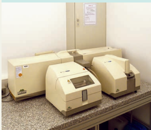
Particle size analyser, Mastersizer 2000, Malvern Instruments Ltd.
