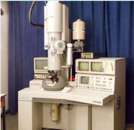
Transmission electron microscope, CM200STEM, Philips
