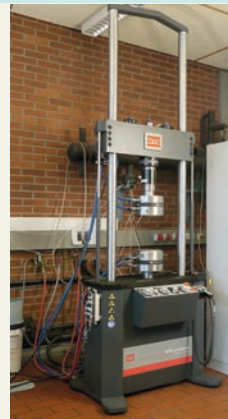
Servo-hydraulic testing system, MTS Landmark, MTS Systems
