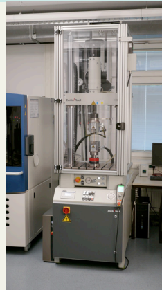
Servo-hydraulic testing machine, Amsler HC 10 Compact, Zwick GmbH & Co. KG
