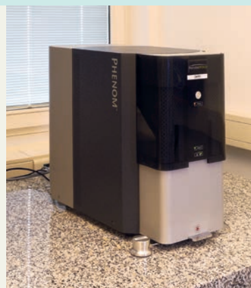
Scanning Electron Microscope (SEM), Phenom SEM, Phenom World
