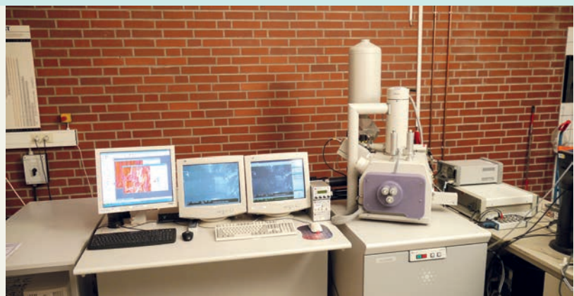
Scanning electron microscope, XL 40 ESM TMP, Philips
