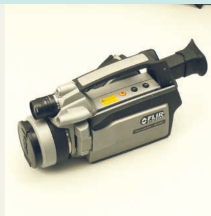
Thermographic camera, P640, FLIR Systems, Inc.
