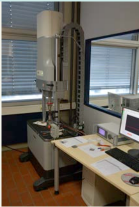
Electrodynamic testing system, ElectroPuls E10000, Instron
