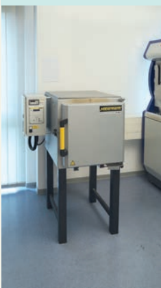
Annealing furnace N30/85HA(-K), Nabertherm GmbH
