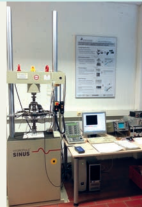
Servo-hydraulic testing system, HYDROPULS SINUS, Schenck
