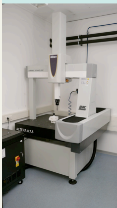
Coordinate Measuring Machine, Nikon Modell "Altera 8.7.6"
