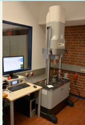
Electrodynamic testing system, ElectroPuls E10000, Instron
