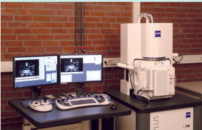
Field Emission SEM, Ultra Plus, Zeiss
