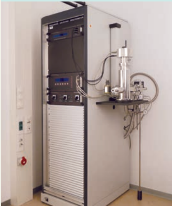
Broadband dielectric spectrometer, Novocontrol GmbH
