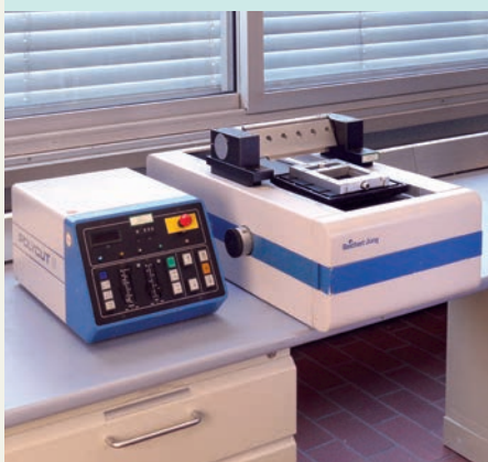
Thin Cutting device, Polycut, Reichert Jung
