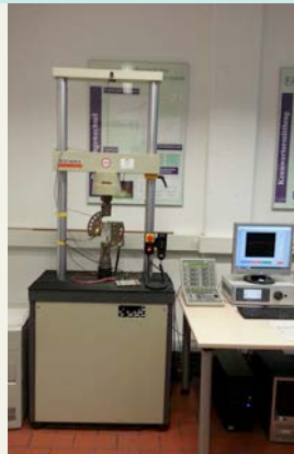
Servo-hydraulic testing system, HYDROPULS, PSA, Schenck
