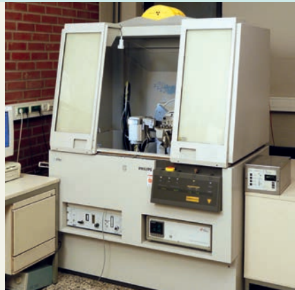
X-Ray diffractometer, X'pert Pro, Philips
