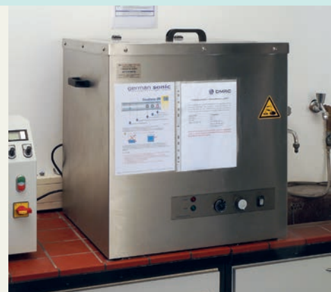
Ultrasonic clean station, UW90, German Sonic Ultraschallanlagen GmbH
