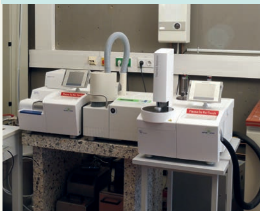
thermoanalytical testing devices, TGA/DSC 1 Star-System + TMA/SDTA841, Mettler Toledo Intl. Inc.
