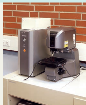
Confocal laser microscope, VK - 9710, Keyence
