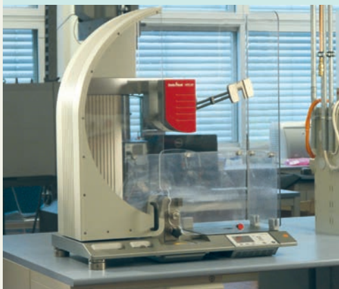
Pendulum impact tester, HIT5.5P, Zwick Roell
