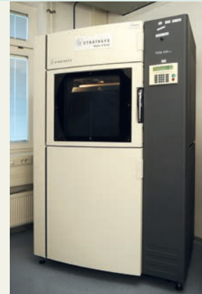
Fused Deposition Modeling Machine, Fortus 400mc, Stratasys
