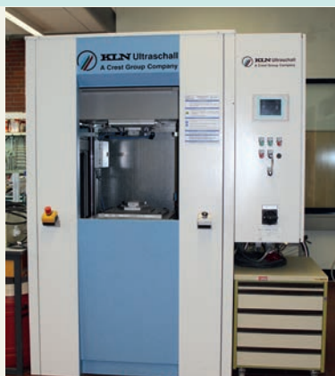
Ultrasonic welding machine, LV 2020-CPC, KLN Ultraschall AG
