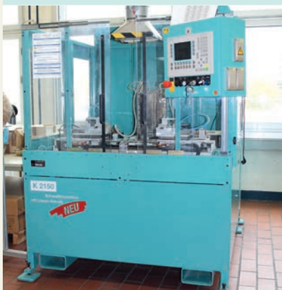
Hot plate welding machine, K2150, Bielomatik Leuze GmbH
