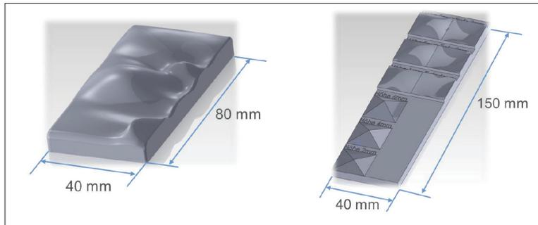
Figure 1: Test specimen geometry for optical measurement systems
