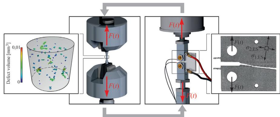
Figure 1: Interaction of fatigue, crack growth and its influencing factors
