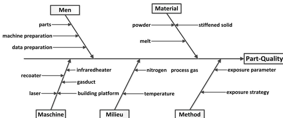
Figure 1: Example of an Ishikawa-diagram for laser sintering
