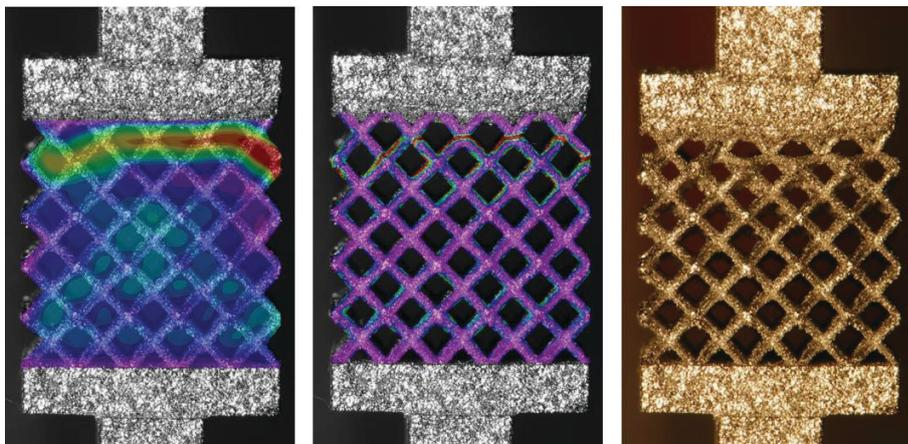
Figure 2: Local strains and sample failure structure in terms of a common sandwich structure featuring bulk face sheets and a lattice core was developed. These tests gave first insights into the structures' capabilities under actual loading conditions.
