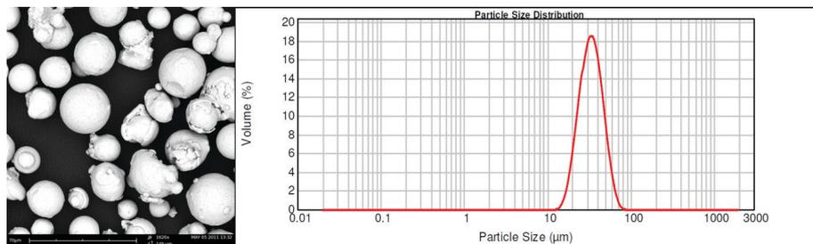
Figure 1: Particle form and size of powder material
