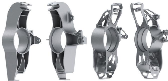
Figure 2: Sample part redesign of a wheelcarrier of the formula student series
