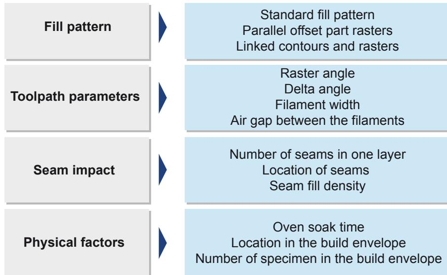
Figure 1: Possible influencing factors on the Z-axis mechanical properties
