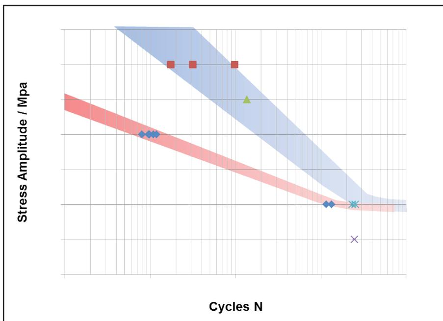
Figure 2: HCF-tests of a Nickel-based superalloy at different temperatures
