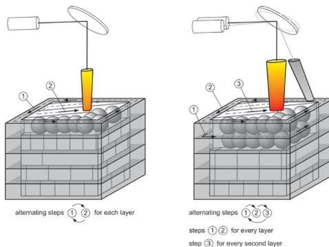
Figure 1: Schematic drawing of different exposure strategies of SLM 250<sup>HL</sup> (left) and SLM 280<sup>HL</sup> (right)
