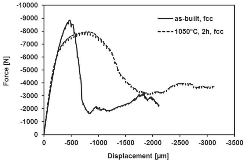
Figure 1: Deformation behavior following SLM and after heat treatment
