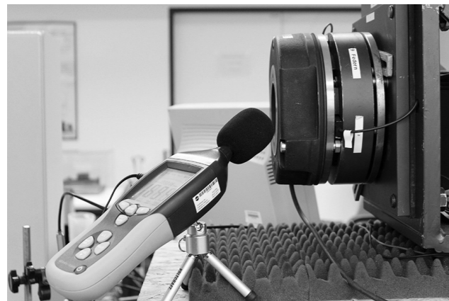
FIGURE 1 Test rig used for sound pressure level tests
