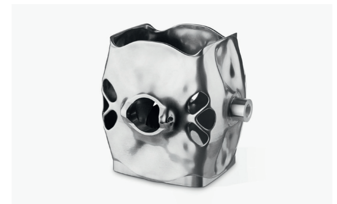
FIGURE 2 Component after final surface finish through vibratory grinding
