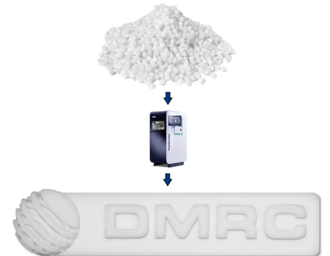
FIGURE 1 Additive production of three-dimensional components from standard plastic granules
