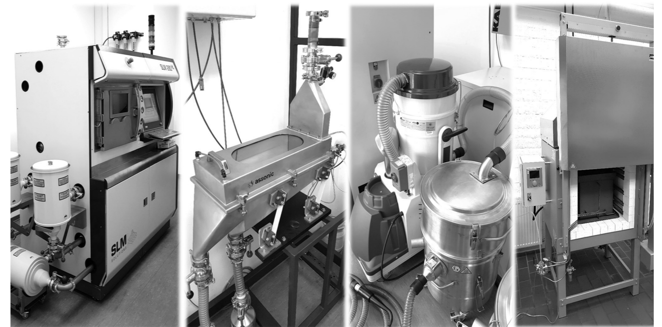
FIGURE 2 Representation of the purchased LBM machine and associated peripheral systems for the LBM process chain
