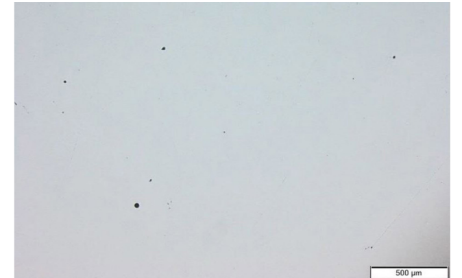
FIGURE 1 Spherical gas porosity
