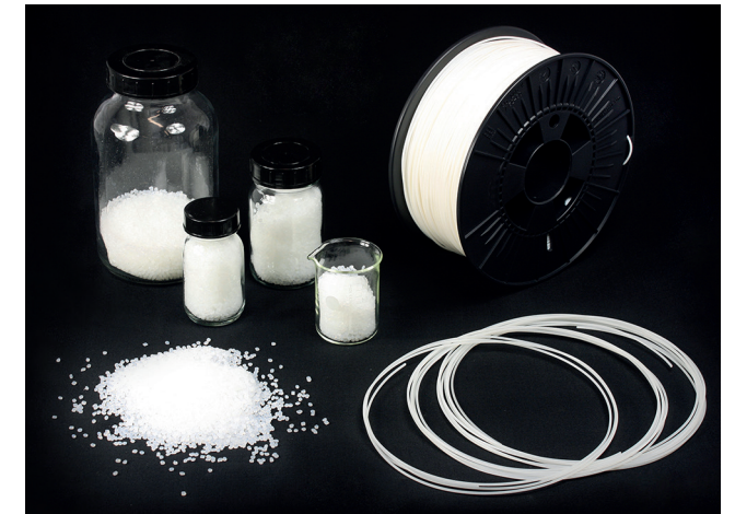
FIGURE 1 Granules and filaments for FDM processing
