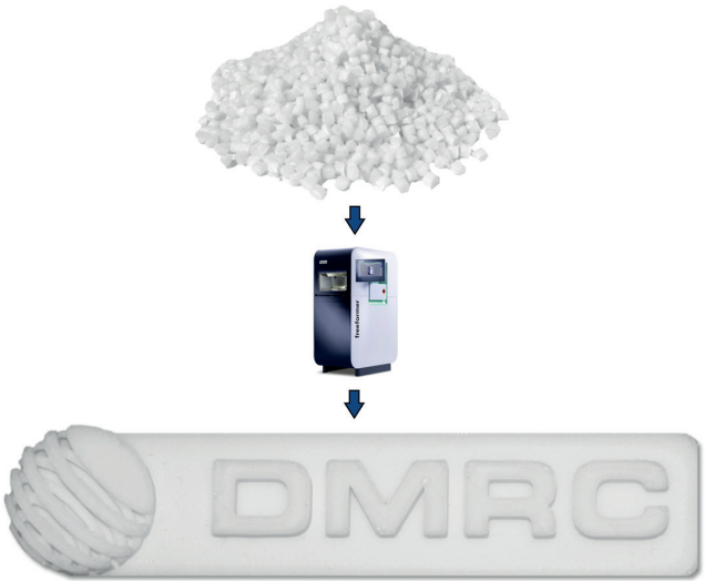
FIGURE 1 Additive production of three-dimensional components from standard plastic granules
