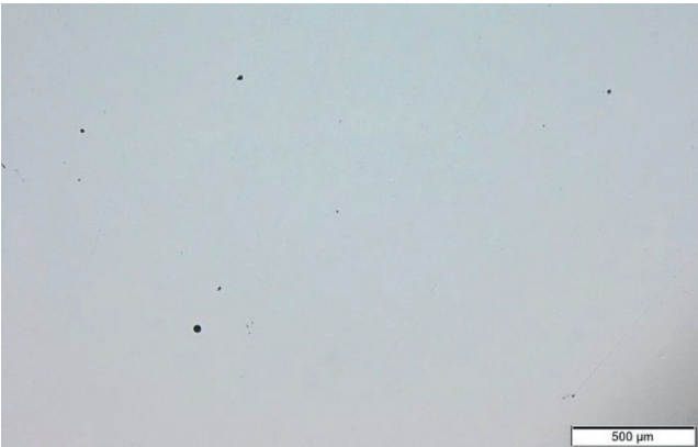
FIGURE 1 Spherical gas porosity
