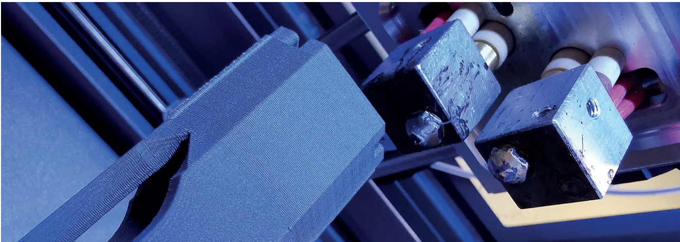
FIGURE 1 FDM part out of a metal powder filled polymer
