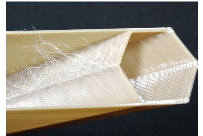
FIGURE 2 Typical FDM error pattern oozing / stringing
