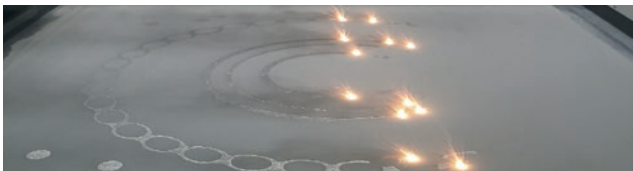
FIGURE 1: Multiple laser interacting with the powder bed (Source: SLM Solutions)
