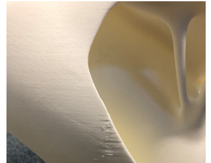
FIGURE 1 Recoater Failure Initiated Part Failure
