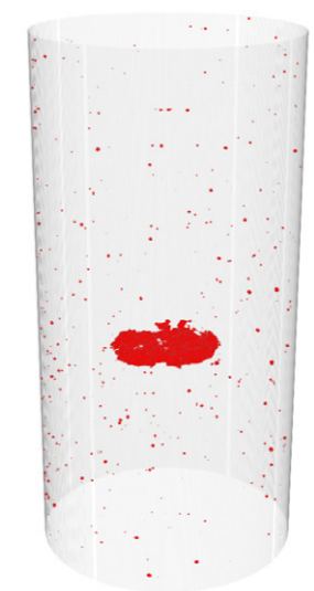
FIGURE 3 Computed tomography scan of Ti6Al4V sample
