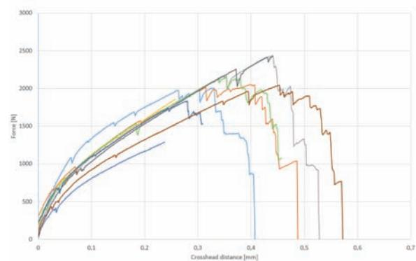
Figure 7: Force-distance diagram of support-structure (block) tensile specimen
