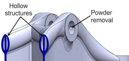
Figure 47: Bracket design with internal structures
