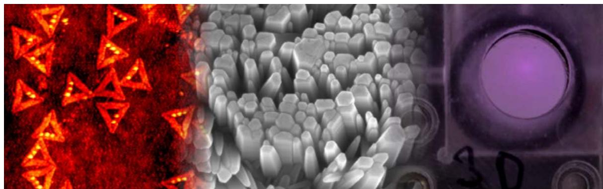
Figure 69: DNA origami nanostructures (left), ZnO nanorods (center), electrochemical cell (right)
