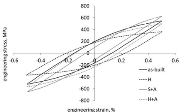
Figure 26: Half-life hysteresis loops for SLM processed IN 718. Tests were carried out at 650 °C with a total strain amplitude of  $\Delta\varepsilon/2 = \pm 0.5\%$
