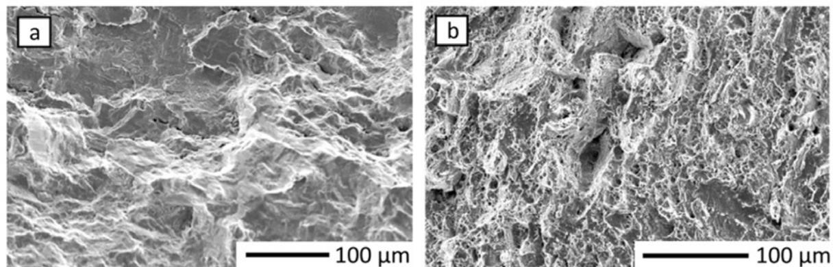
Figure 27: SEM images of the fracture surfaces after LCF testing ( $\Delta\varepsilon/2 = \pm 0.35\%$ ) at 650 °C in the as-built (a) and H (b) condition. The images were taken from the fracture surface showing instable crack growth
