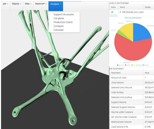
Figure 35: ReactionWheel bracket in the KnowAM-Software Tool
