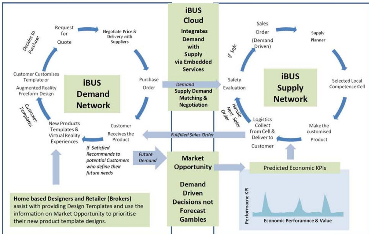
Figure 29: Non-linear supply chain model for demand-driven safe and affordable customised products
