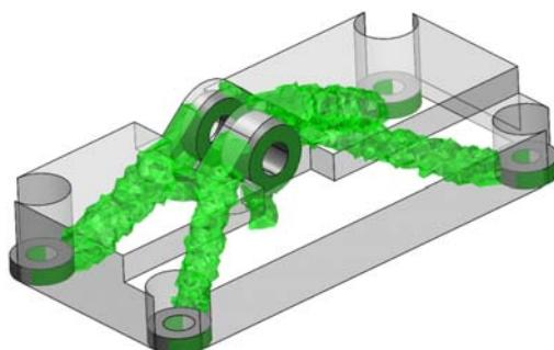
Figure 46: Topology Optimization of the bracket
