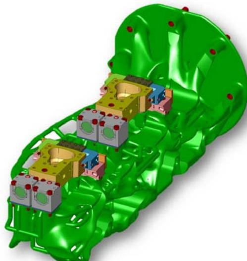
Figure 49: Topology optimized clamping device
