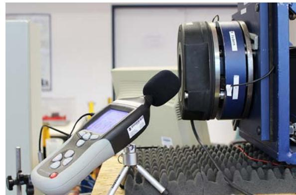
Figure 50: Test rig used for sound pressure level tests
