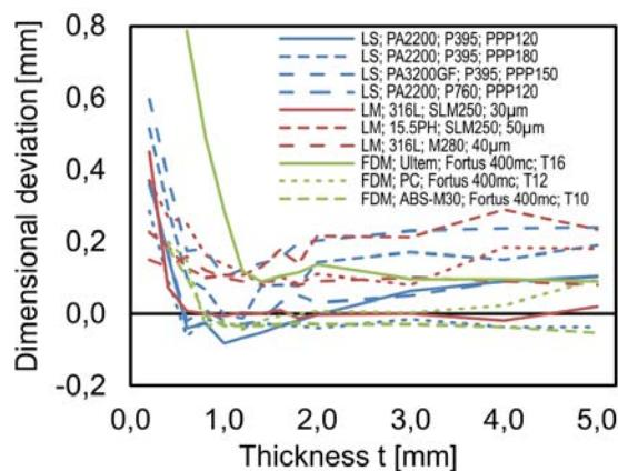
Figure 12: Dimensional deviations for walls manufactured with different thicknesses and boundary conditions
