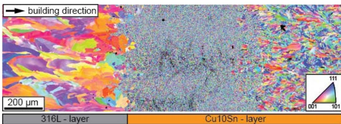
Figure 67: Color-coded orientation map of the functional graded multi-material consisting of 316L and Cu10Sn at an interface area.
